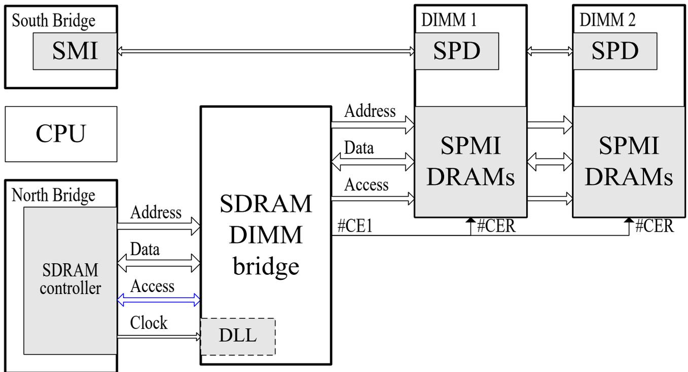
SDRAM DIMM Bridge Board: hardware platform of X86 personal computer
