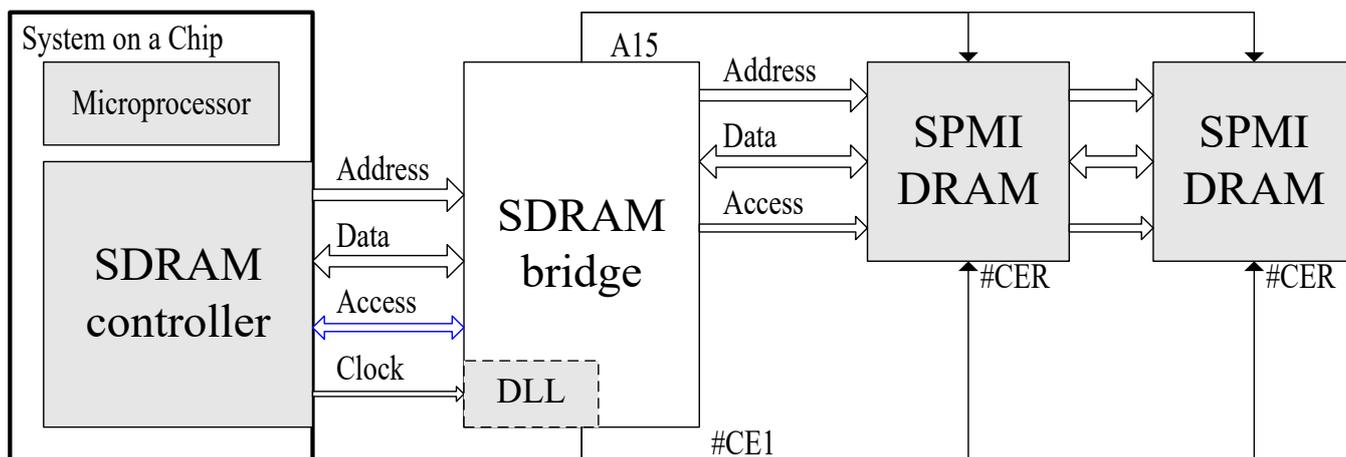
SDRAM DIMM Bridge: hardware platform of X86 personal computer
