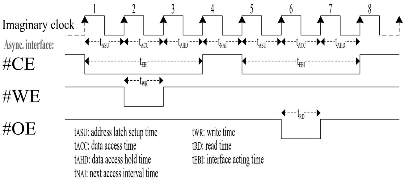
$$t_{EBI} = t_{ASU} + t_{ACC} + t_{AHD}$$
